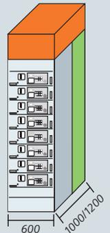
Maloperation protection prevents travel of the withdrawable-units when the master switch is "ON"
